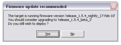
**Note:** To reduce the risk of compatibility problems, we recommend that all the hardware devices (NioNodes, nControl nodes etc.) on the network run the same firmware version, and that the version matches the version of NWare you are running.
